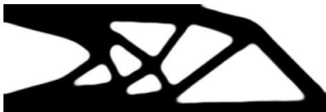
Fig. 3: Optimal design considering the load P , with u_{lim} = 1.50 u_0 . Final volume fraction 49.04%.
