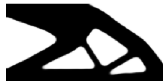
Fig. 5: Optimal design considering the load Q , with u_{lim} = 1.50 u_0 . Final volume fraction 50.38%.
