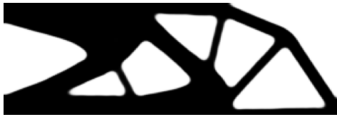
Fig. 6: Optimal design considering the load P and Q as two load cases, with u_{lim,i} = 1.50 u_{0,i} for i = 1, 2 . Final volume fraction 51.42%.
