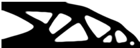
Fig. 7: Optimal design considering the load p , with u_{lim,i} = 1.50 u_{0,i} \forall i . Final volume fraction 53.43%.
