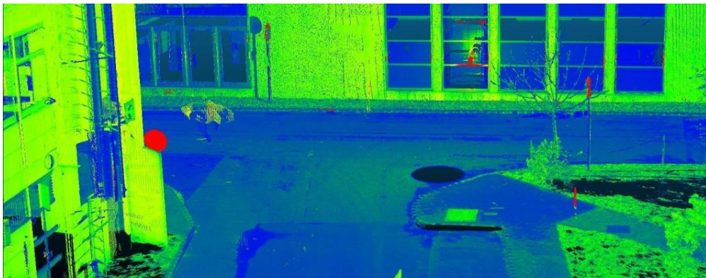
Fig. 3 Terrestrial laser scanner modelled intersection
