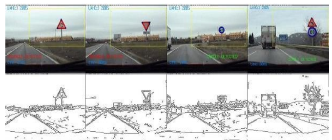
Fig. 3. Real images sequence, detected on the road, with the search area within each image outlined (square window), and Canny image used for contour information search. [7]
