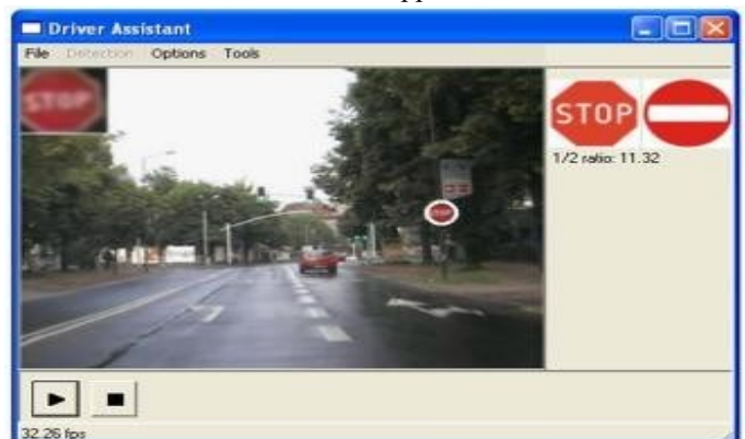
Fig 5. The process of traffic sign recognition shown in a screenshot. The appeared candidates represent the best obtained scores. [25]
