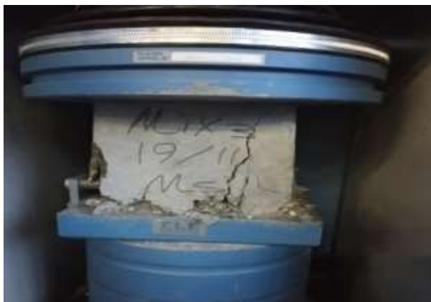
Fig. 3. Compressive strength test in progress [8]
