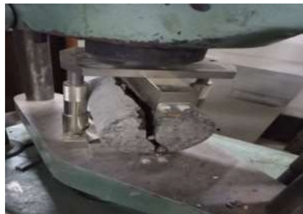
Fig. 5. Splitting tensile strength test in progress [8]
