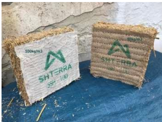
Fig. 1. Shterra thermal insulation straw blankets [13].
