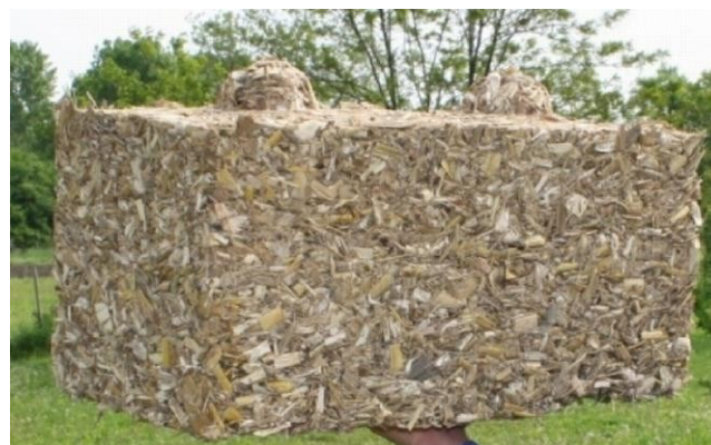
Fig. 2. Cornstalk insulation block [17].
