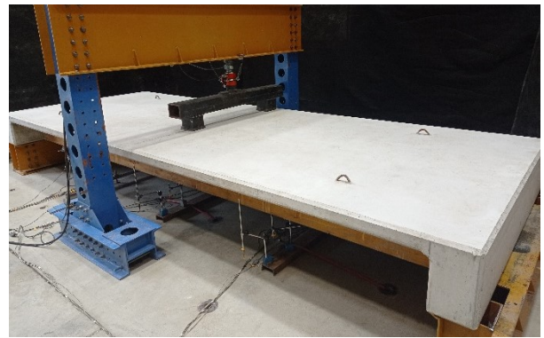
Fig. 7. Axle load arrangements during concentrated load (S_2)
